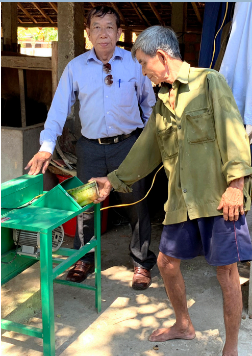
A local farmer illustrates use of a grinding machine. These will be instrumental in grinding agricultural bi-products and forage such as banana trunks into animal feed.
